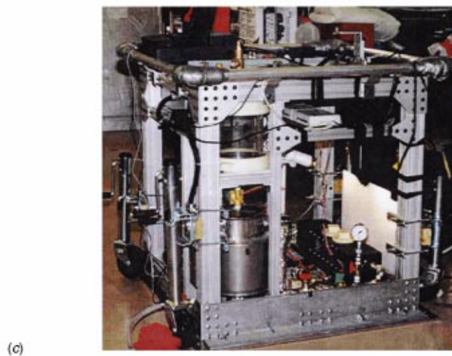
Fig. 1 (a) Schematic, (b) test section, and (c) the photo of the Particle-Melting-in-Flow (PMF) flight test module
